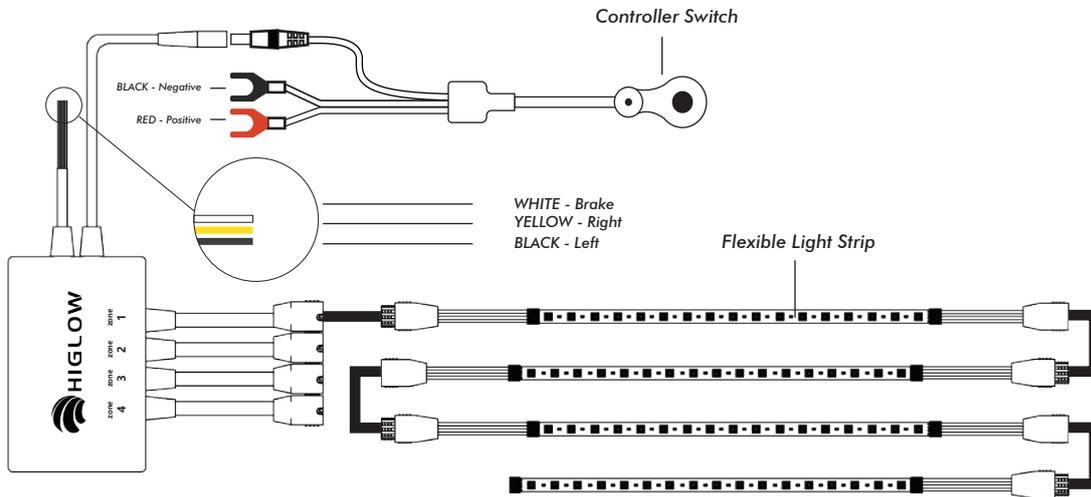
**Step 2 Controller installation** Place the controller around the main driver's seat is suggested. Connect the driving, braking, and steering wires on the controller to the corresponding automobile wiring harness assembly. Pass the switch wires through the engine compartment then connect with the positive and negative of battery. (Note: This step should be performed by relevant professionals).
