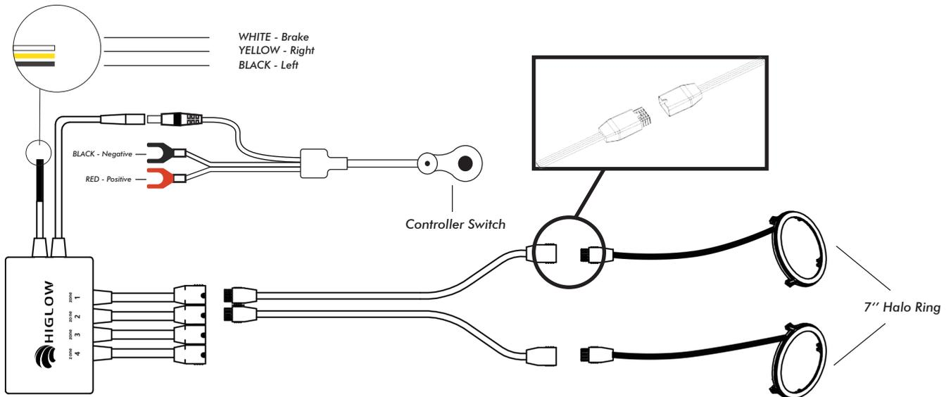
**Step 2 Controller installation** Place the controller around the main driver's seat is suggested. Connect the driving, braking, and steering wires on the controller to the corresponding automobile wiring harness assembly. Pass the switch wires through the engine compartment then connect with the positive and negative of battery. (Note: This step should be performed by relevant professionals).
